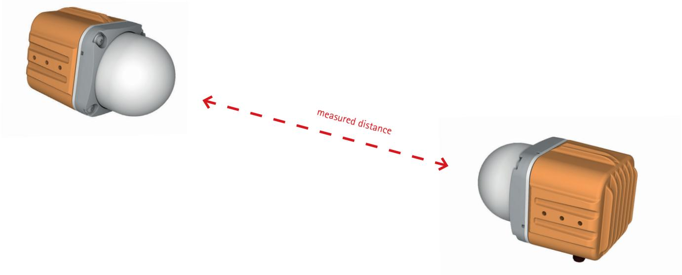
In secondary radar mode two LPR®-1DHP-290 measure the distance and speed between each other. The secondary radar mode features high ranges of up to 300 m and high update rates and ensures that the measurement is taken only to the partner unit. Typical applications are positioning of cranes and heavy machinery, process automation and collision avoidance.
