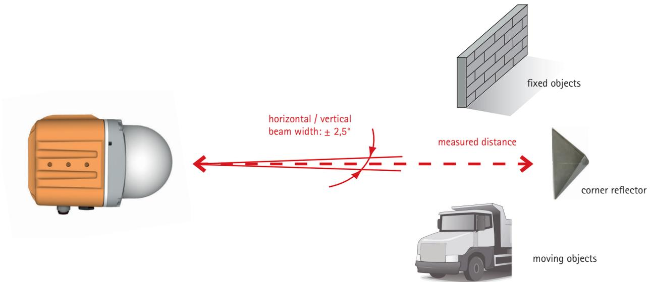
In primary radar mode a single LPR®-1DHP-290 measures the distance and speed to a reflective object, typically a metal corner reflector. The range is typically 50 m but depends on the radar cross section (RCS) of the used target. The primary radar mode features very high update rates and enables a cost effective installation. Typical applications are positioning of cranes and heavy machinery, presence check, level probing and detection of objects.
